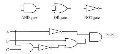
Figure 1.3: The standard symbols for the three basic logic gates, and a logic circuit that computes the value of the logical expression  $(\neg A) \land (B \lor \neg (A \land C))$ . The input wires to each logic gate are on the left, with the output wire on the right. Note that when wires cross each other in a diagram such as this, the wires don't actually intersect unless there is a black circle at the point where they cross.
