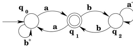
Next we note that there is in fact a loop from  $q_1$  to  $q_1$  via  $q_0$ . A regular expression that matches the strings that would move around the loop is  $ab^*a$ . So we add a transition labeled  $ab^*a$  from  $q_1$  to  $q_1$ , and remove the now-irrelevant  $a$ -transition from  $q_1$  to  $q_0$ . (It is irrelevant because it is not part of any other loop from  $q_1$  to  $q_1$ .)
