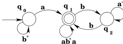
Next we note that there is also a loop from  $q_1$  to  $q_1$  via  $q_2$ . A regular expression that matches the strings that would move around the loop is  $ba^*b$ . Since the transitions in the loop are the only transitions to or from  $q_2$ , we simply remove  $q_2$  and replace it with a transition from  $q_1$  to  $q_1$ .
