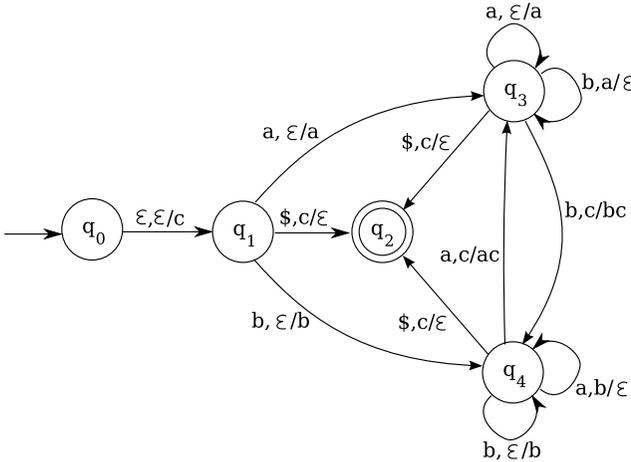
In this modified automaton, it is only possible for the machine to reach the accepting state  $q_2$  by reading the end-of-string symbol at a time when the number of  $a$ 's that have been consumed is equal to the number of  $b$ 's. Taking our cue from this example, we define what it means for a language to be deterministic context-free as follows:
