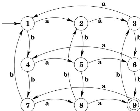
Consider the sequence of states that the machine passes through while processing the string  $abbbabb$ . Note that there is a repeated state (state 2). We say that  $abbbabb$  “goes through the state 2 twice”, meaning that in the course of the string being processed, the machine is in state 2 twice (at
