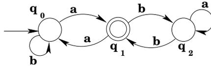
Note that there is a loop from state  $q_2$  back to state  $q_2$ : any number of  $a$ 's will keep the machine in state  $q_2$ , and so we label the transition with the regular expression  $a^*$ . We do the same thing to the transition labeled  $b$  from  $q_0$ . (Note that the result is no longer a DFA, but that doesn't concern us, we're just interested in developing a regular expression.)
