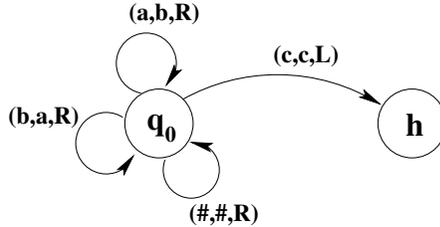
To simplify the diagrams, I will leave out any transitions that are not relevant to the computation that I want the machine to perform. You can assume that the action for any omitted transition is to write the same symbol that was read, move right, and halt.
