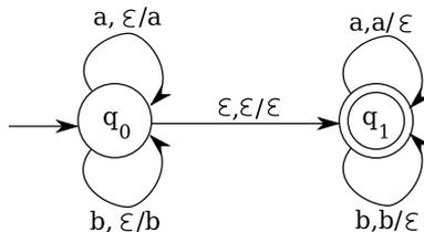
In state  $q_0$ , this machine copies the first part of its input string onto the stack. In state  $q_1$ , it tries to match the remainder of the input against the
