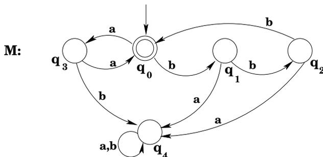
The start state of  $M$  is accepting, which means  $\varepsilon \in L(M)$ . If  $M$  is in state  $q_0$ , a sequence of two  $a$ 's or three  $b$ 's will move  $M$  back to  $q_0$  and hence be accepted. So  $L(M) = L((aa \mid bbb)^*)$ .
