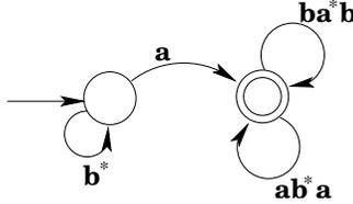
It is now clear from the diagram that strings of the form  $b^*a$  get you to state  $q_1$ , and any number of repetitions of strings that match  $ab^*a$  or  $ba^*b$  will keep you there. So the machine accepts  $L(b^*a(ab^*a \mid ba^*b)^*)$ .
