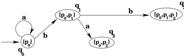
The construction continues as long as there are new states being added, and new transitions from those states that have to be computed. The final DFA is shown below.
