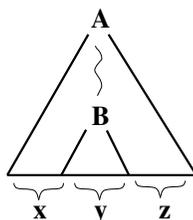
represents a parse tree in which the yield is the string  $xyz$ . The string  $y$  is the yield of a smaller tree, with root  $B$ , which is contained within the larger tree. Note that any of the strings  $x$ ,  $y$ , or  $z$  could be the empty string.
