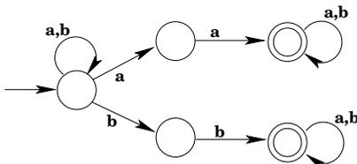
3. Give a DFA that accepts the language accepted by the following NFA. (Be sure to note that, for example, it is possible to reach both  $q_1$  and  $q_3$  from  $q_0$  on consumption of an  $a$ , because of the  $\varepsilon$ -transition.)
