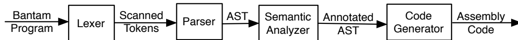
Figure 1: Bantam Java compiler phases. Note: AST is short for Abstract Syntax Tree.
