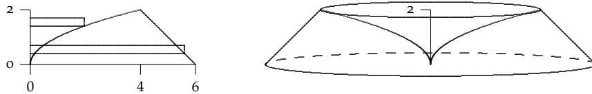
Figure 6.18: Left: The region enclosed by the curves y = \sqrt{x} , y = 6 - x , and the x -axis and two representative rectangles. Right: The resulting solid of revolution about the x -axis (a ‘volcano’) is formed by two distinct pieces each requiring its own integral.
