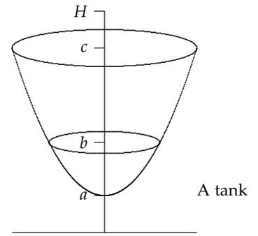
containing a liquid between levels  $a$  and  $b$ . The top of the tank is at height  $c$ . The liquid is to be moved to a height  $H$  above the tank.
