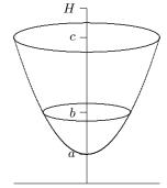
A tank containing a liquid between levels a and b. The top of the tank is at height c. The liquid is to be moved to a height H above the tank.
